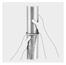
**Mounts quickly without standpipe cap** No standpipe cap is needed thanks to the perfectly fitting transition.
