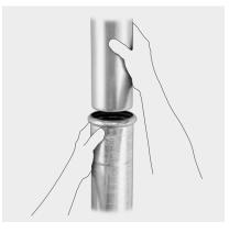
Just insert Insert rainwater downpipe into the standpipe's long-sleeve socket.
