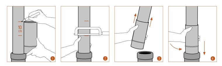
● Simply mark downspout at the height of the siphon trap, mark again 10 cm below. ② Cut the pipe at the bottom mark. While doing this, hold the pipe piece firmly to avoid its slipping into the stand pipe and then remove. ③ Slide the siphon trap over the downspout which is bent to the side. ④ Swivel downspout back again and push the siphon trap in up to the end stop groove in the stand pipe.
